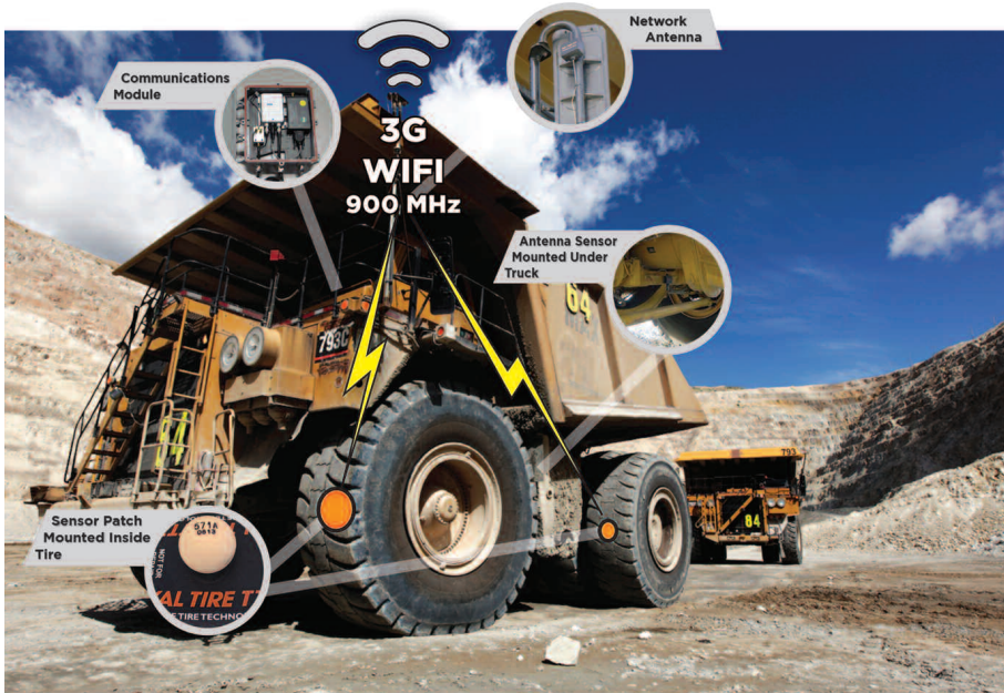
TTT installation elements on customer mining truck
