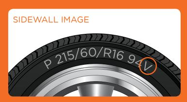
The last letter of the tire size on the sidewall of your tire indicates the 'speed rating'— how fast your tires can travel for a certain length of time. But it's not just about speed. Speed rating is an indication of a tire's performance—how your tires get rid of heat and how they brake, corner, grip and swerve just in time.
