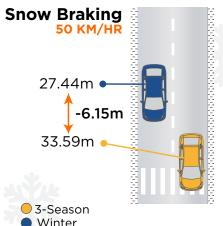
Air temperature during testing was +1.5°C
