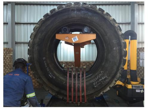
Above: Pressure and heat are applied to ensure that repairs are able to seal fully with the tire. Right: Damaged tires are carefully prepared by expert Kal Tire staff prior to repairs being installed.
