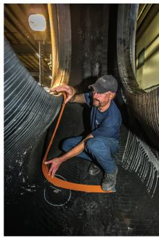
Clockwise from top left: Damaged areas of the tire are cut out; damaged steel bands are repaired and replaced; rubber patches designed to match the contour of the tire are applied, and later heated for proper curing; damage to the face of tires is filled with new rubber, which is cut to match the existing tread pattern later.
